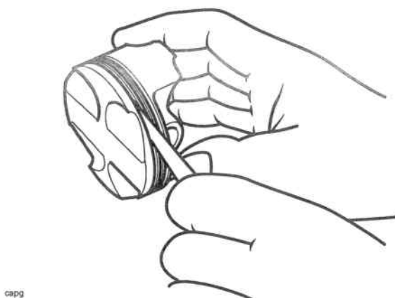
Piston Ring to Ring Groove Clearance Check
